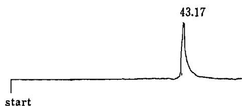
Fig. 8. Elution of Synthetic \alpha -rCGRP from a TSKgel G 2000SW Column ( 7.5 \times 600 mm)
